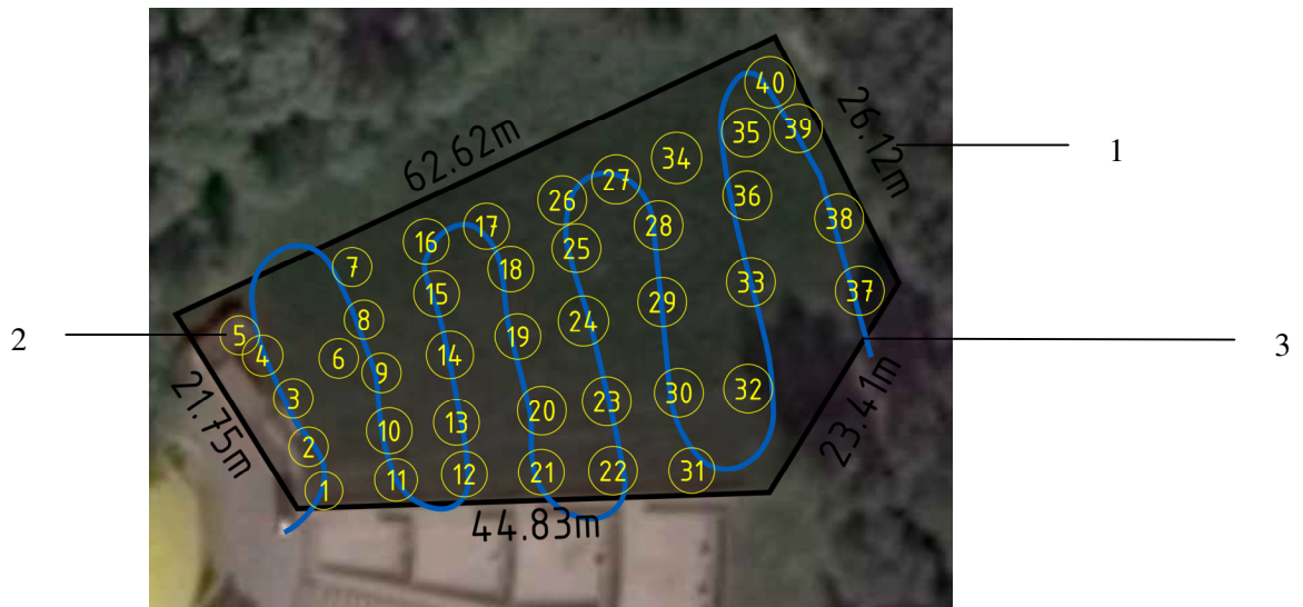
Fig. 1. Object of study: 1 – sizes of the object; 2 – ground control points; 3 – flight strips
